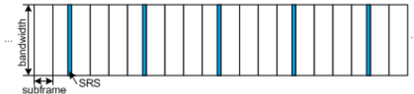
SRS transmission with frequency hopping ( B_{\text{SRS}} \neq 0 )
